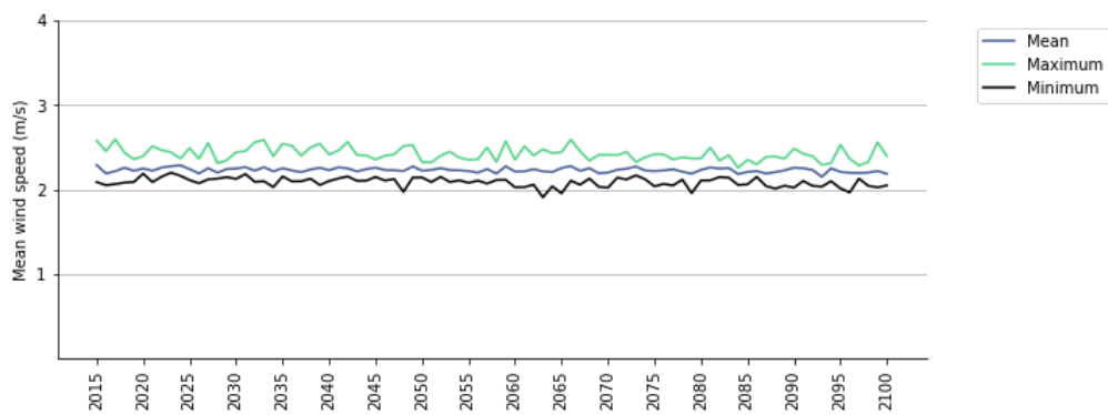
Figure 60. Ensemble mean annual daily wind speed and range of variation (Maximum and Minimum) for a set of six models in the SSP585 scenario (2015-2100) for Trentino.
